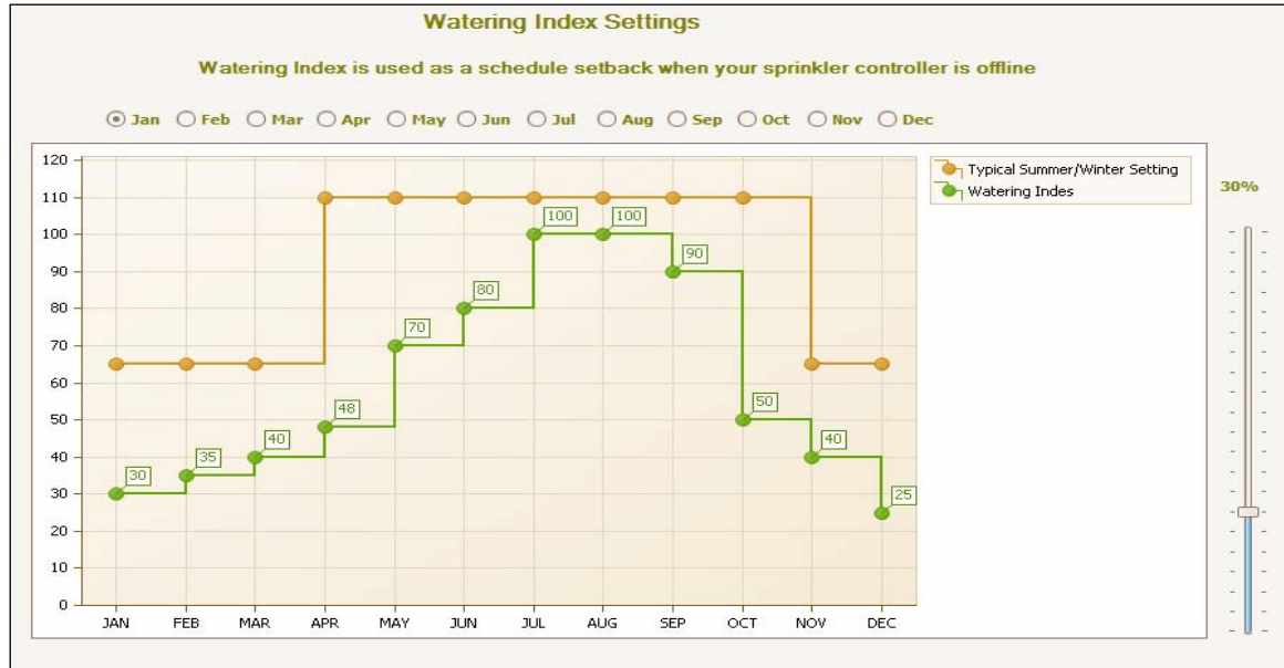
Figure 6 - Cyber-Rain Watering Index settings example
