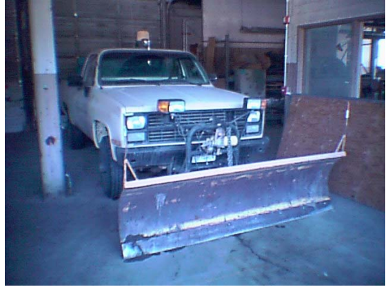
Pickup truck with blade. (source: Tahoe Truckee Unified School District)
