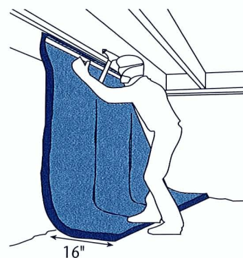
Figure 15: Nail long pieces of insulation to the band joist.
