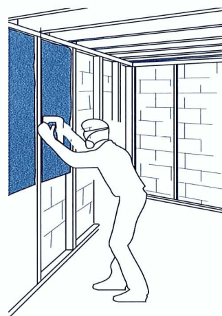
Figure 16: Cut insulation to extend from the top plate to at least 2 feet below ground level.
