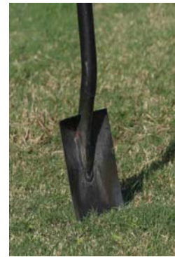
Figure 6. Square point ditching shovel required for SMS installation.
