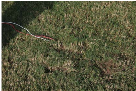
Figure 19. Soil and turfgrass plug replaced, covering SMS prior to burying wire.
