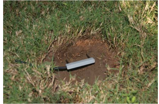
Figure 21. LawnLogic SMS partially inserted into turfgrass root zone of undisturbed soil.
