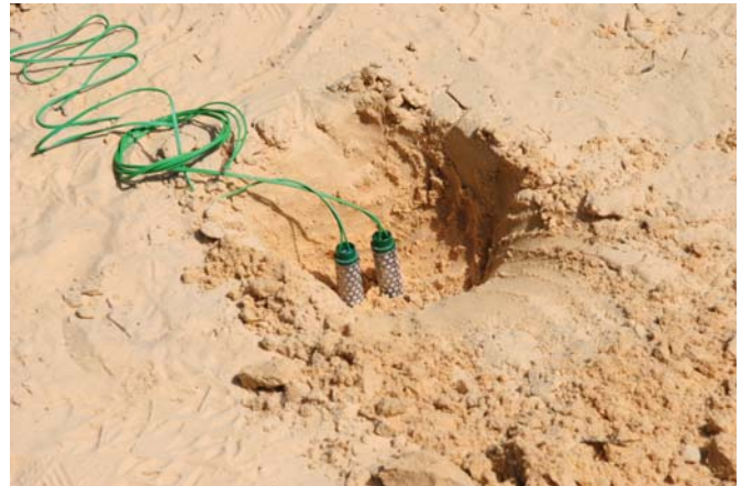
Figure 20. Irrrometer Watermark SMS being installed in a new landscape.
