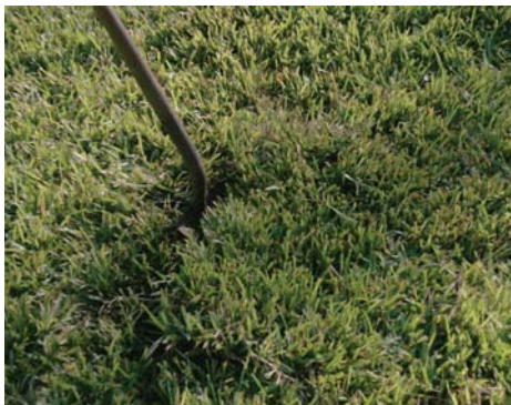
Figure 10. Cutting a square of turfgrass large enough to cover entire probe.
