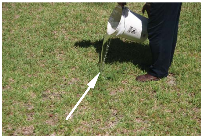
Figure 38. Establishing the controller set-point—bucket method. Arrow points to sensor location.
