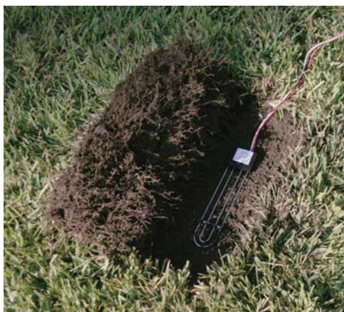
Figure 12. SMS installed in root zone by "roll back" method.
