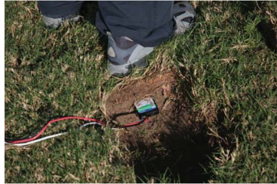
Figure 18. Compaction of soil around sensor to reduce void space and ensure adequate connection between SMS and soil.
