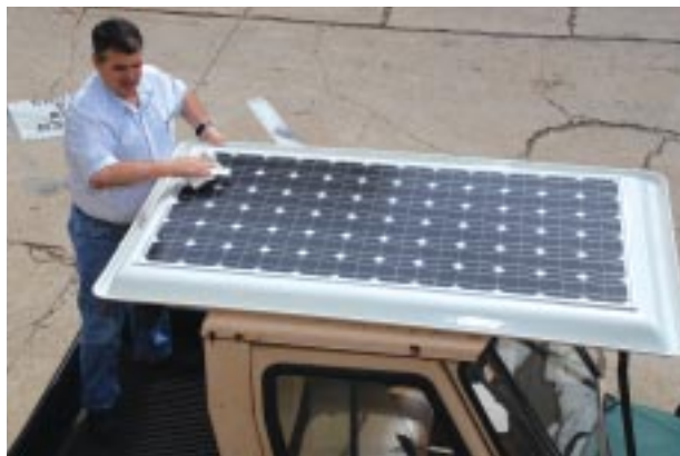
Environmental engineer Mark Weir cleans the solar cell panel of the FRCSW Environmental Program Office's electric cart which was recently augmented with solar power. The solar conversion is expected to gain a 30 percent increase in distance from a single battery charge.
