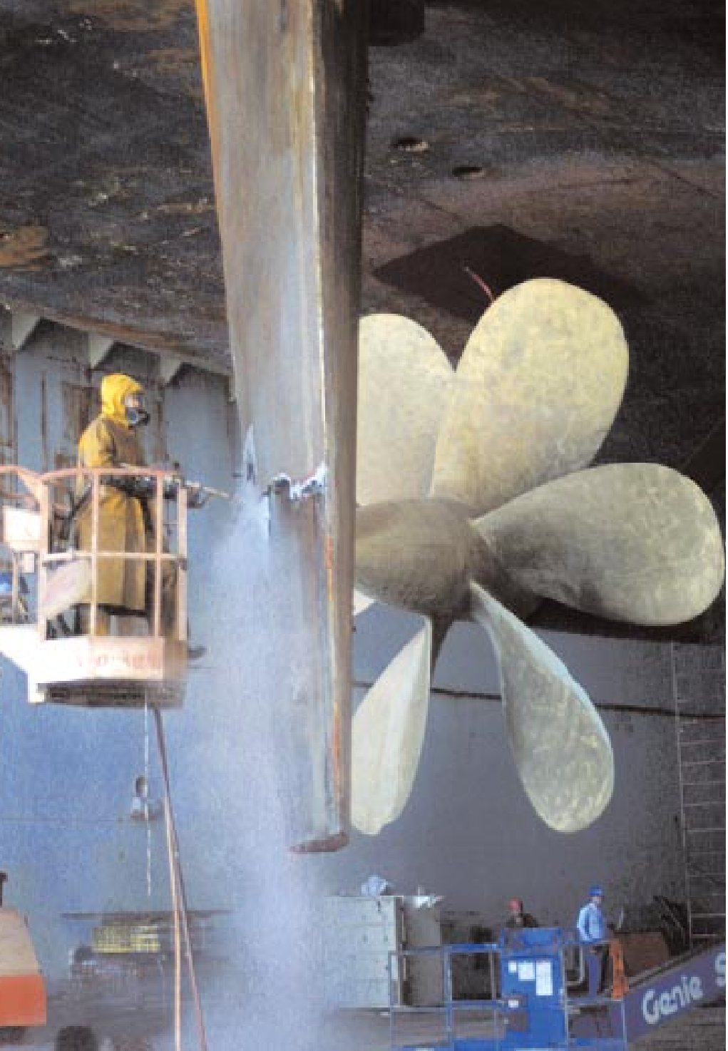
Regular barnacle removal and hull cleaning contributes to a reduced lifespan for the ship. Photographer's Mate 3rd Class Erika Jones
