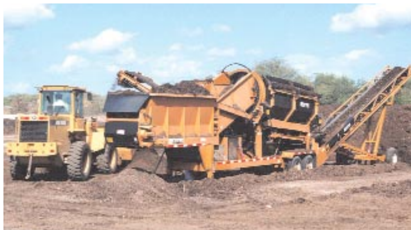
A trommel screen sifts composted material at NAVFAC Hawaii's Biosolids Treatment Facility, Kalaeloa, Oahu. Denise Emsley
