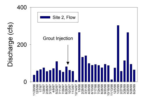
**Figure 2.** Flow rates from the main seep (Site 2) at the Roberts-Dawson mine before and after grouting. The arrow indicates the approximate date in which grouting of FGD began.
