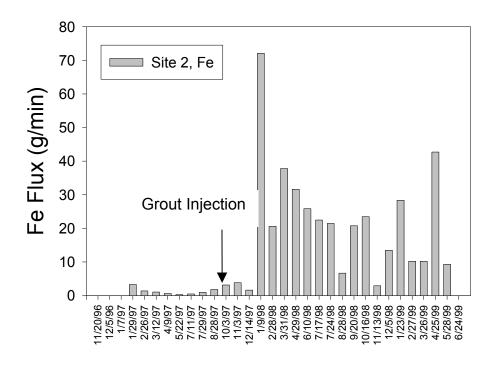
**Figure 3.** Flux of iron from the main seep (site 2) at the Roberts-Dawson Mine before and after grouting. The arrow indicates the approximate date in which grouting of FGD began.
