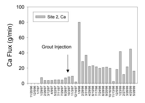
**Figure 4**. Flux of calcium from the main seep (site 2) at the Roberts-Dawson mine before and after grouting. The arrow indicates the approximate date in which grouting of FGD began.
