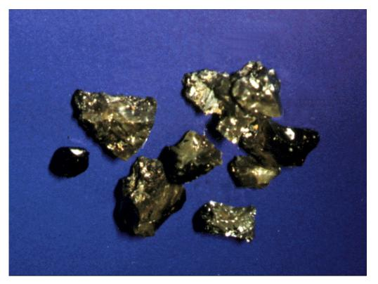
Fig.1 The plasma vitrified product for 50/50% mixture of bottom ash coming from medical waste incineration and fly ash coming from the power plant
