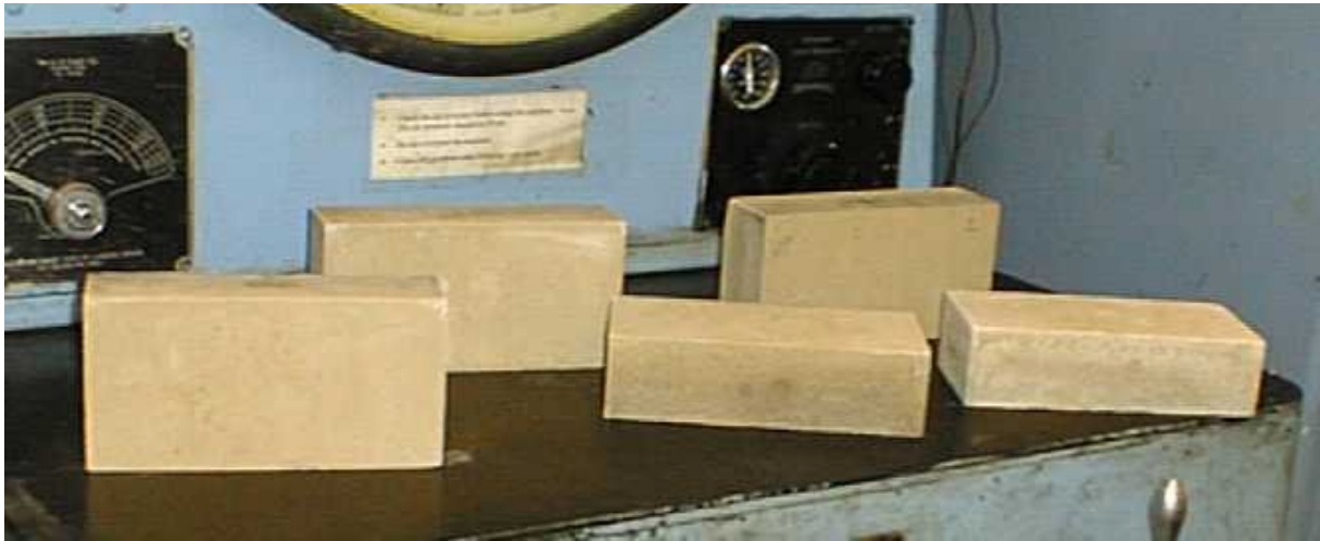
Figure 1. Fly ash bricks compacted in laboratory by using a Baldwin Hydraulic Press. (Note that the fly ash used for the bricks shown in the above photo is high-grade Class C fly ash.)
