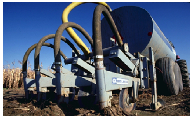
Figure 5. Sub-surface application of liquid manure on land using a slurry tank with injection toolbar to reduce ammonia volatilization.
