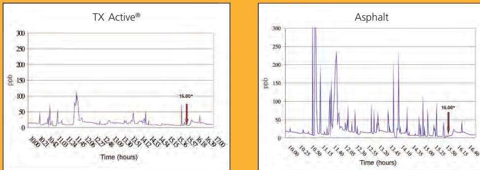
\*For the purpose of appraising the reproducibility and reliability of the testing instrumentation, at 4.00 p.m. both analyzers were placed in the area paved with photoactive blocks with data being acquired for about an hour.
