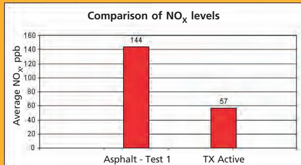
Based on recorded data, up to 60% NO<sub>x</sub> abatement was achieved compared to the untreated area, depending on luminous intensity, traffic volume, as well as wind speed and direction. The best results were obtained in summer with an average luminous intensity of about 90,000 Lux, a wind speed of approximately 0.7 m/s, an ambient temperature of 32°C, and 46% humidity.
