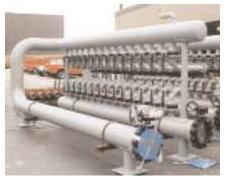
5. Header plumbing before being installed in valve pit.
