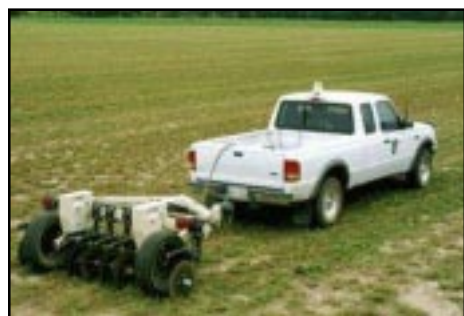
GPS-equipped vehicle performing EC mapping passes (Veris Technologies, Salina, KS).
