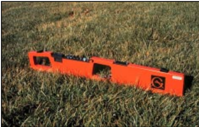
Non-contact sensor using EM to measure soil EC (USDA-ARS Photo Gallery, Columbia, MO).
