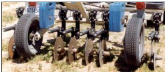
Coulter-mounted electrodes need soil contact to measure EC (USDA-ARS Water Management Unit, Ft. Collins, CO).
