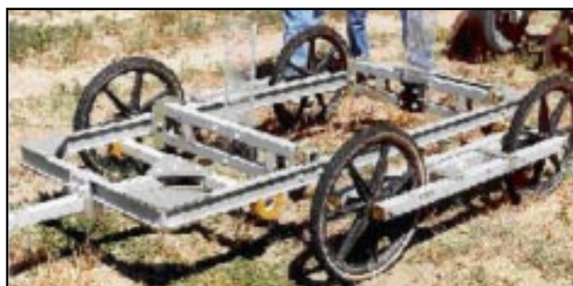
Non-metallic cart used for transporting non-contact EMI sensor (USDA-ARS Water Management Unit, Ft. Collins, CO).
