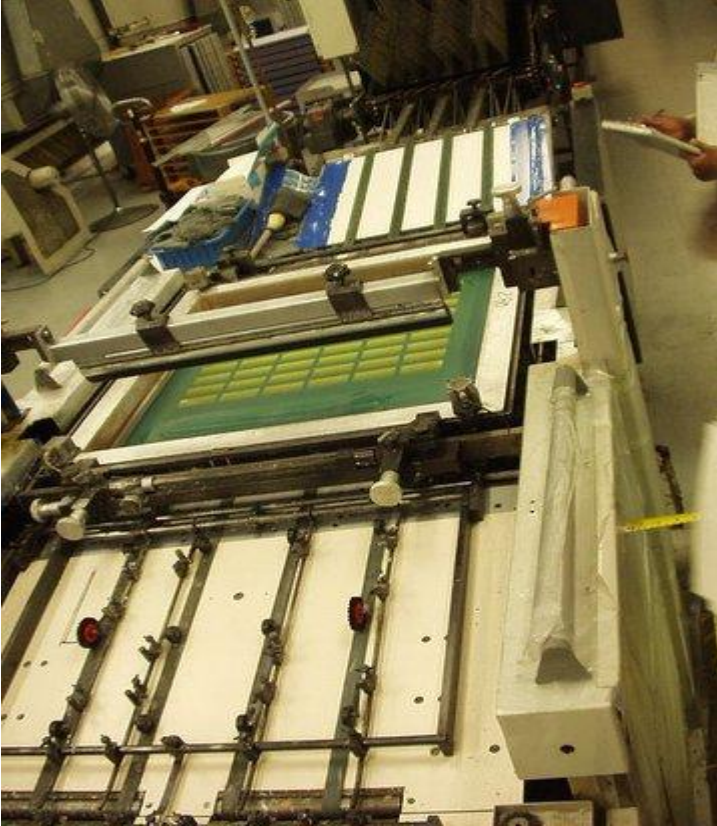
Figure 2-3. Automated Printing Press at Oberthur
