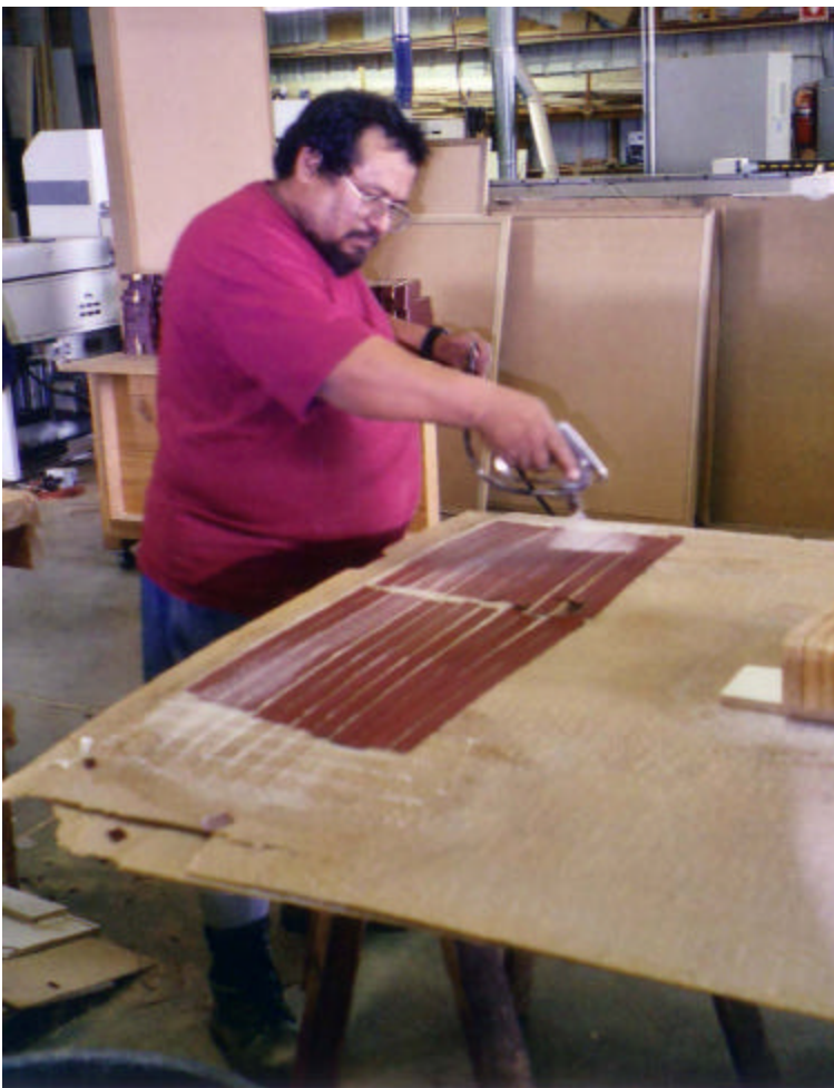
Figure 2-12 Applying New Adhesive at United Cabinet Company
