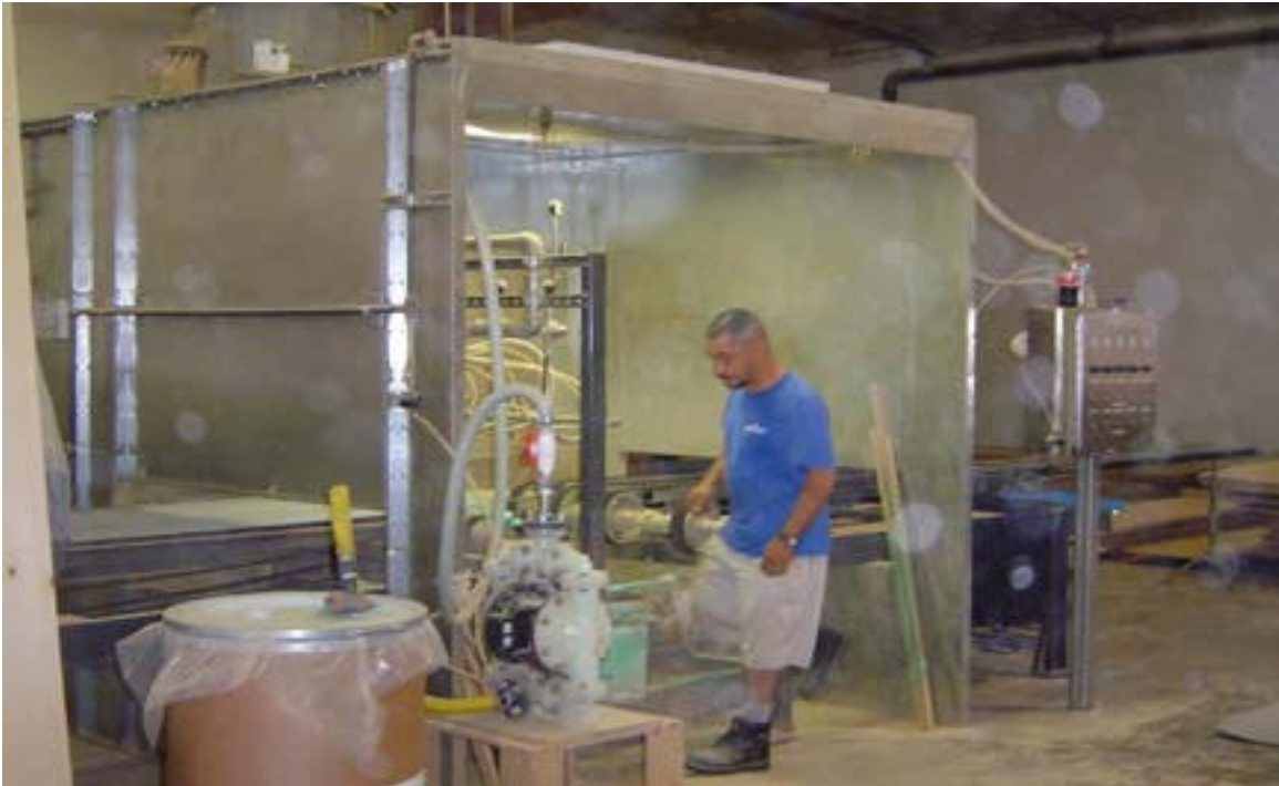
Figure 2-10 Adhesive Line at The Countertop Factory
