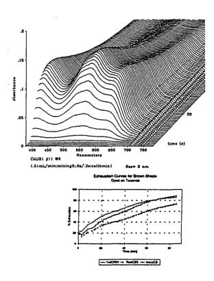
repeated on fabric samples dyed in a laboratory Texomat. The exhaustion curves from these experiments were much smoother, which substantiated the idea that machine noise was the primary cause of noise in the package machine exhaustion curves.
