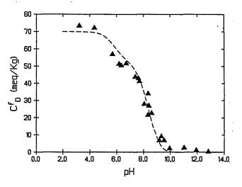
analyze data for the equilibrium uptake of C.I. Acid Blue 45 by nylon 6. A good non-linear fit of the experimental data, based on the measured acidic and basic end group contents of the fibers, was obtained from the dimensionless model, as can be seen in the Figure. The dimensionless parameters were estimated while fitting the data to the dimensionless model. On
