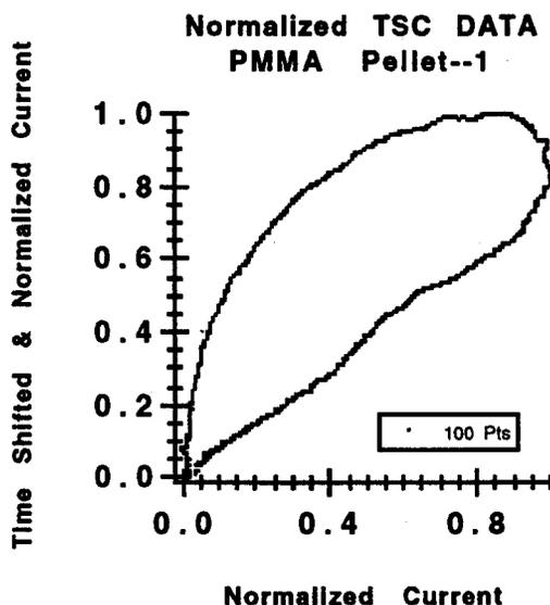
Figure 6a) Phase space portrait of PMMA pellet
