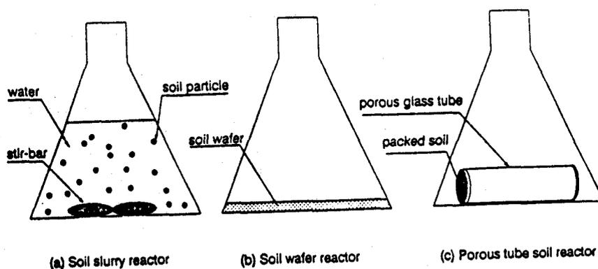
FIGURE 1 Schematic of Soil Slurry, Soil Wafer and Soil Porous Tube Respirometric Reactors
