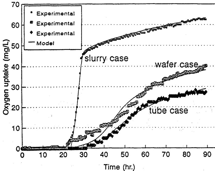
FIGURE 2 Oxygen Uptake Curves for Soil Slurry, Wafer and Porous Tube Reactors for Phenol. The line indicates the Fit by the Mathematical Model Developed for each Reactor Type
