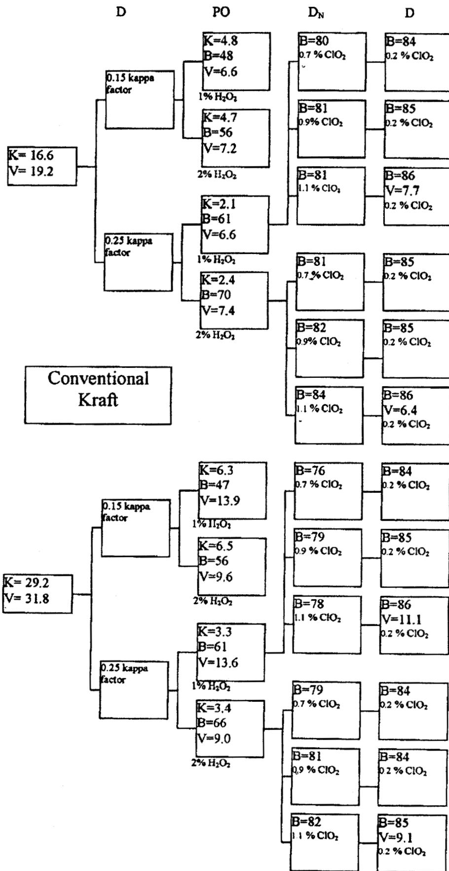
Figure 3: Results from D(PO)DND for conventional kraft pulp
