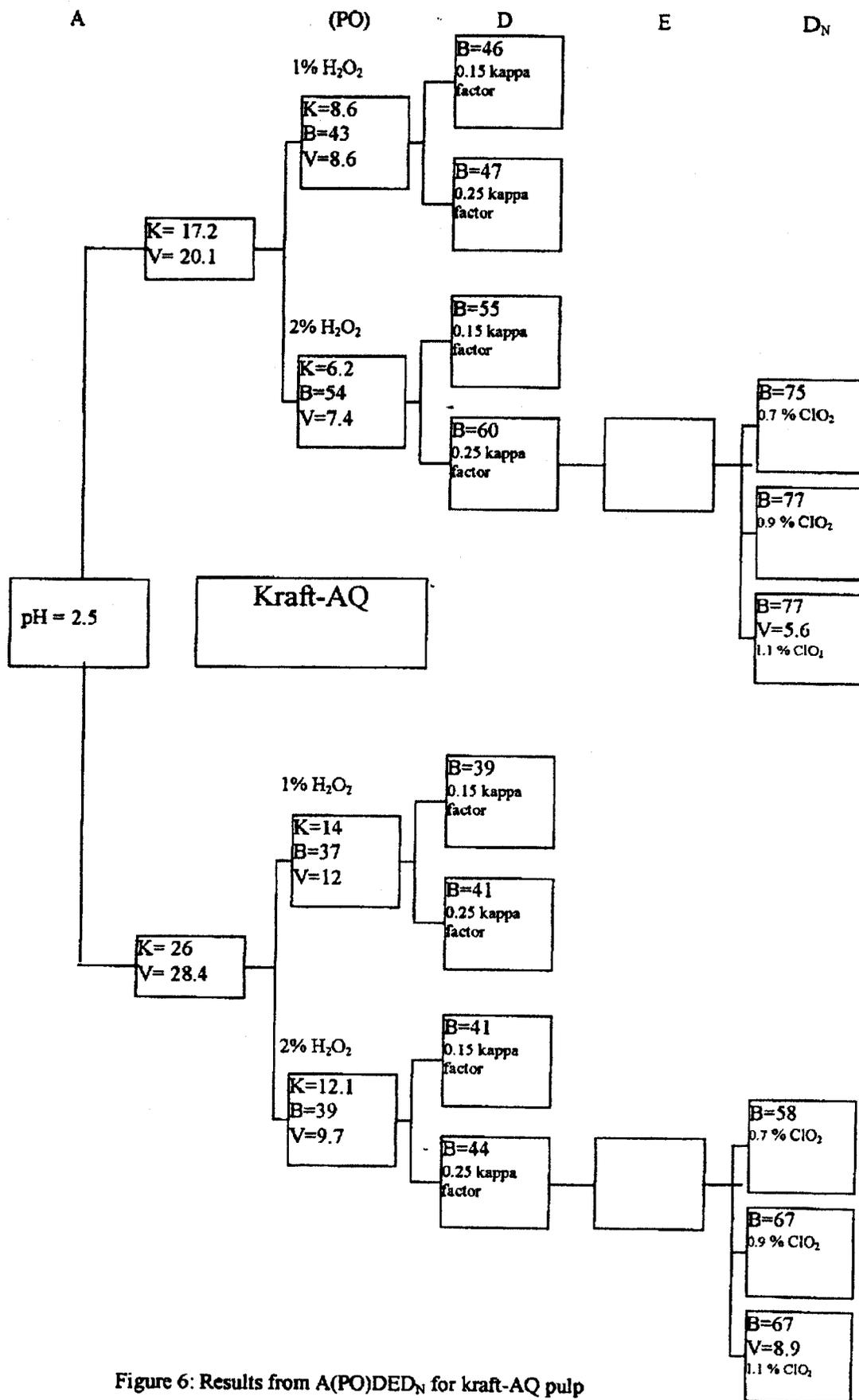
Figure 6: Results from A(PO)DED<sub>N</sub> for kraft-AQ pulp
