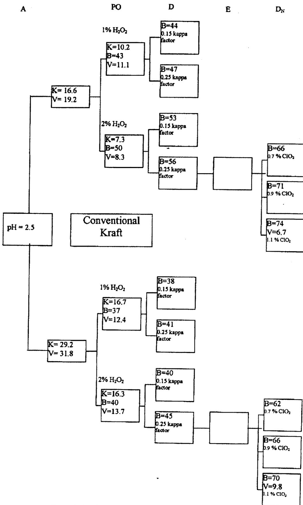
Figure 5: Results from A(PO)DED<sub>N</sub> for conventional kraft pulp
