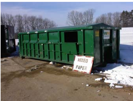
Side loading roll-off container for mixed paper, Concord Drop-Off, Concord
