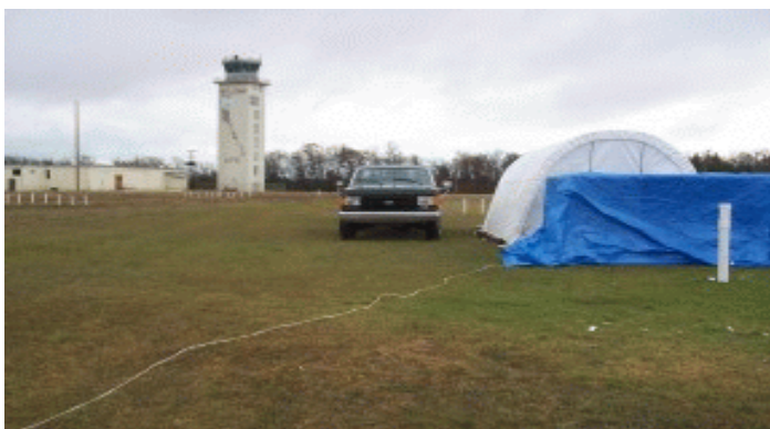
Experimental lanes at the MIRTL. The MIRTL is a controlled release facility in which natural- and controlled-gradient, in-situ groundwater experiments can be conducted.
