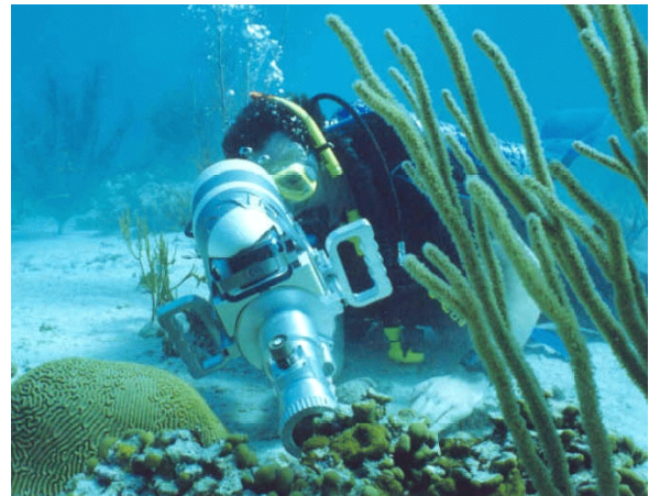
Non-destructive assessment of the health of benthic photosynthetic organisms using an underwater FRR fluorometer.
