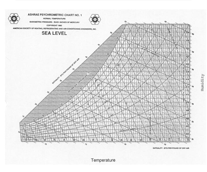
Engineering tool to calculate the energy in moist air
