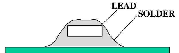
Solder does not flow over top of foot on Pd plated leads
