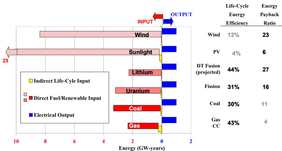
Two metrics are considered in this study: Life-Cycle Efficiency (LCE) and Energy Payback Ratio (EPR). LCE (Equation 1) is the ratio of the useful electrical output to the sum of the thermal input of fuel supplied both at the plant and throughout the life-cycle.
