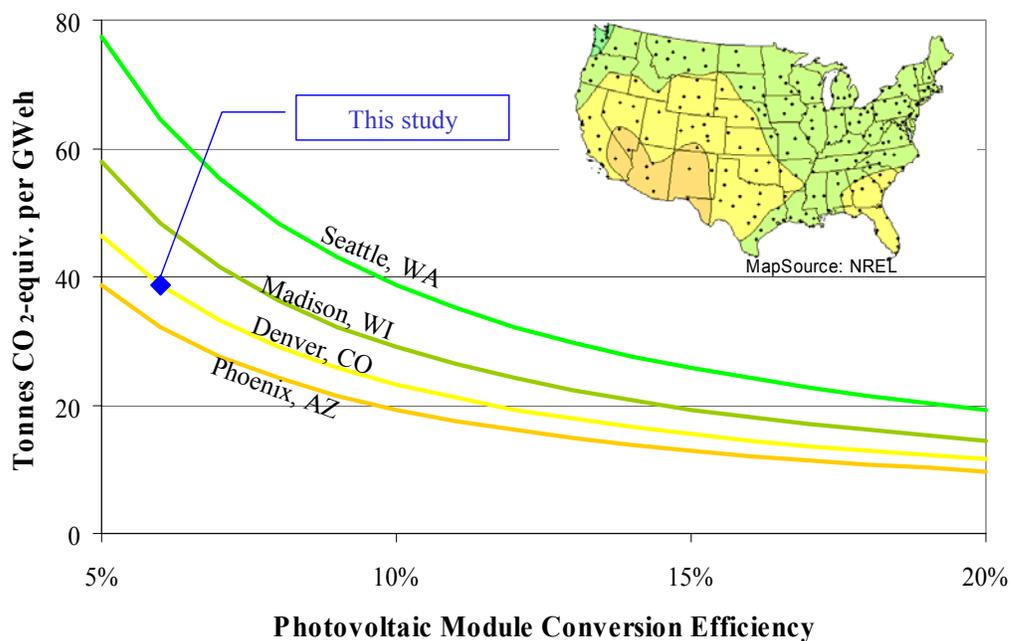
**Figure 31: PV greenhouse gas emission rate decreases in the future based on improvements in the conversion efficiency.**
