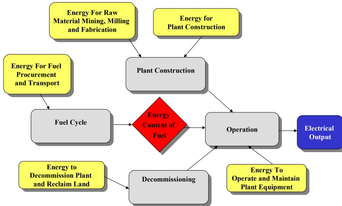
For a natural gas plant, the output energy is a simple calculation based on the average electrical power output of the plant, average capacity factor, and plant lifetime. The output energy for the PV system may be based on actual performance data, or estimated using the average solar insolation rate and the module conversion efficiency.
