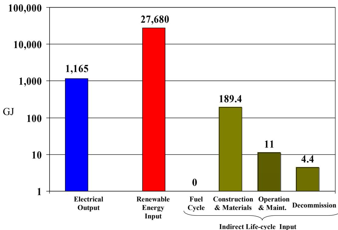
Figure 19: Conventional Module Conversion Efficiency and Life-Cycle Efficiency for an 8 kW Thin Film PV System
