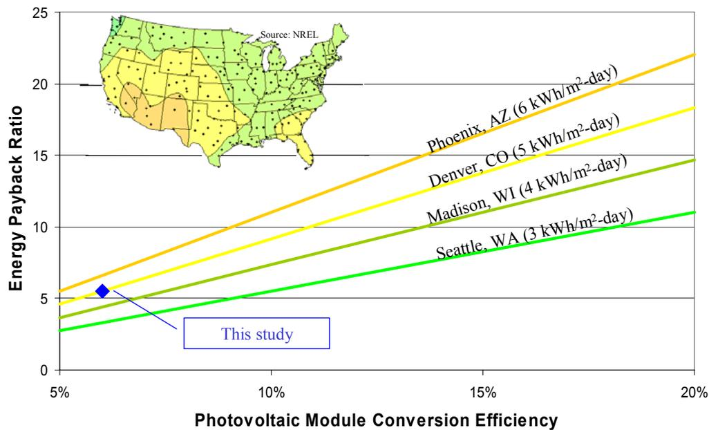
Figure 25: Future improvements in conversion efficiency (9-20%) increase the photovoltaic EPR to between 8 and 18.
