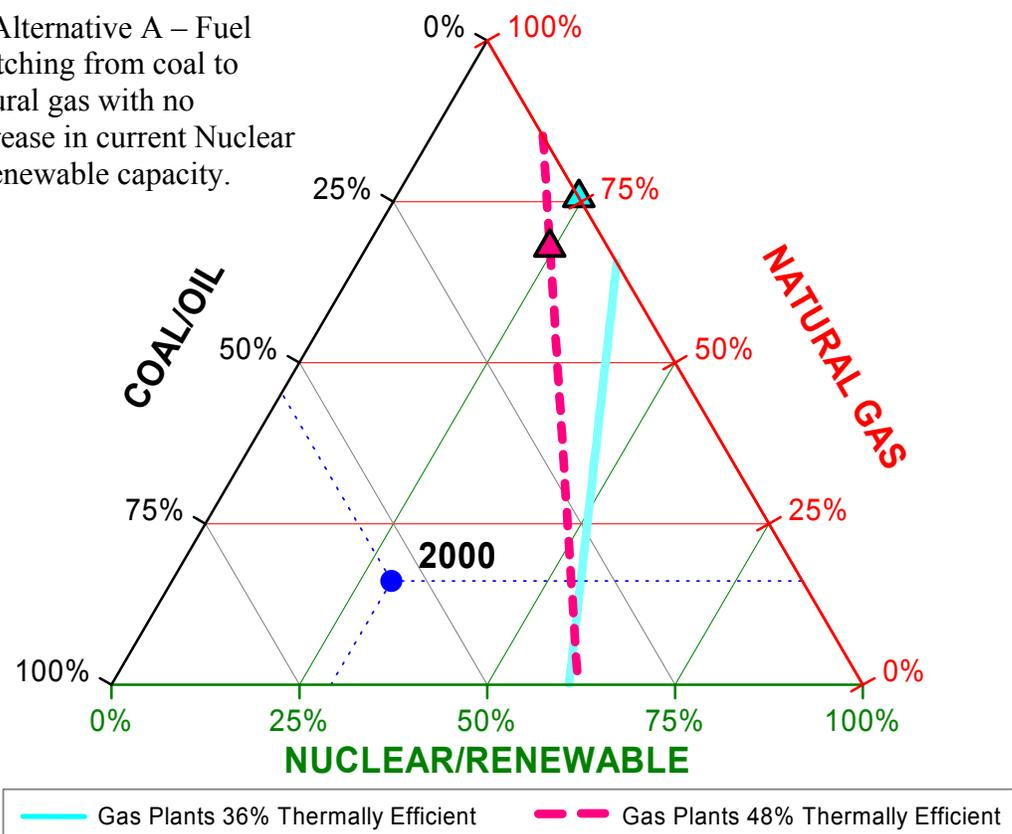
**Figure 37: Implementing Alternative A with high efficiency natural gas requires an 83% replacement of coal generation to meet a Kyoto-based emission target.**
