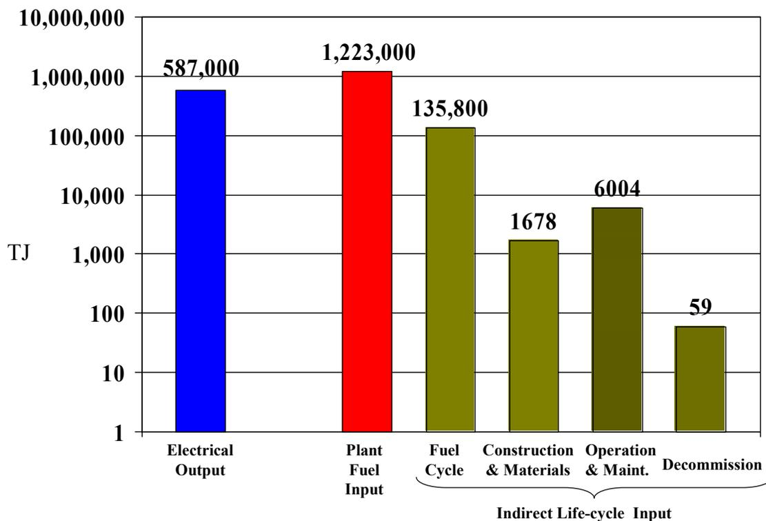
**Figure 16: Conventional Plant Efficiency and Life-Cycle Efficiency for the Combined-Cycle Natural Gas Plant**
