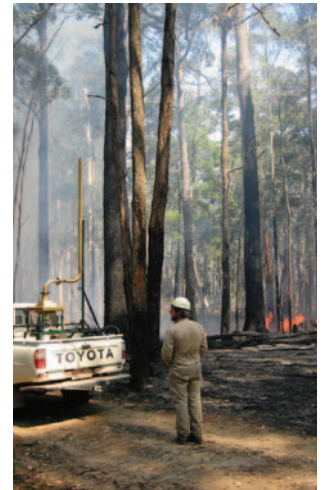
A pump is used to collect smoke samples during a prescribed burn. Photo by C Meyer.
