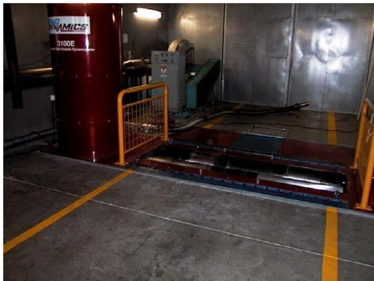
*Figure 3.2: Dyno Dynamics Chassis Dynamometer inside the test cell looking rearward towards the vehicle entry doors*
