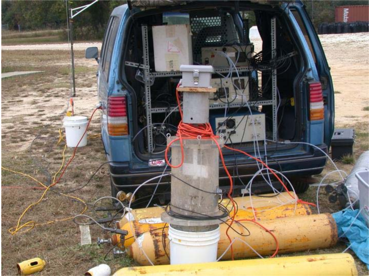
Figure 4.10. Dynamic flow-through chamber system mounted on 5 gallon plastic bucket. Modification in measurement protocol was necessary to successfully measure ammonia flux from the porous, heterogeneous material in the composting bins.
