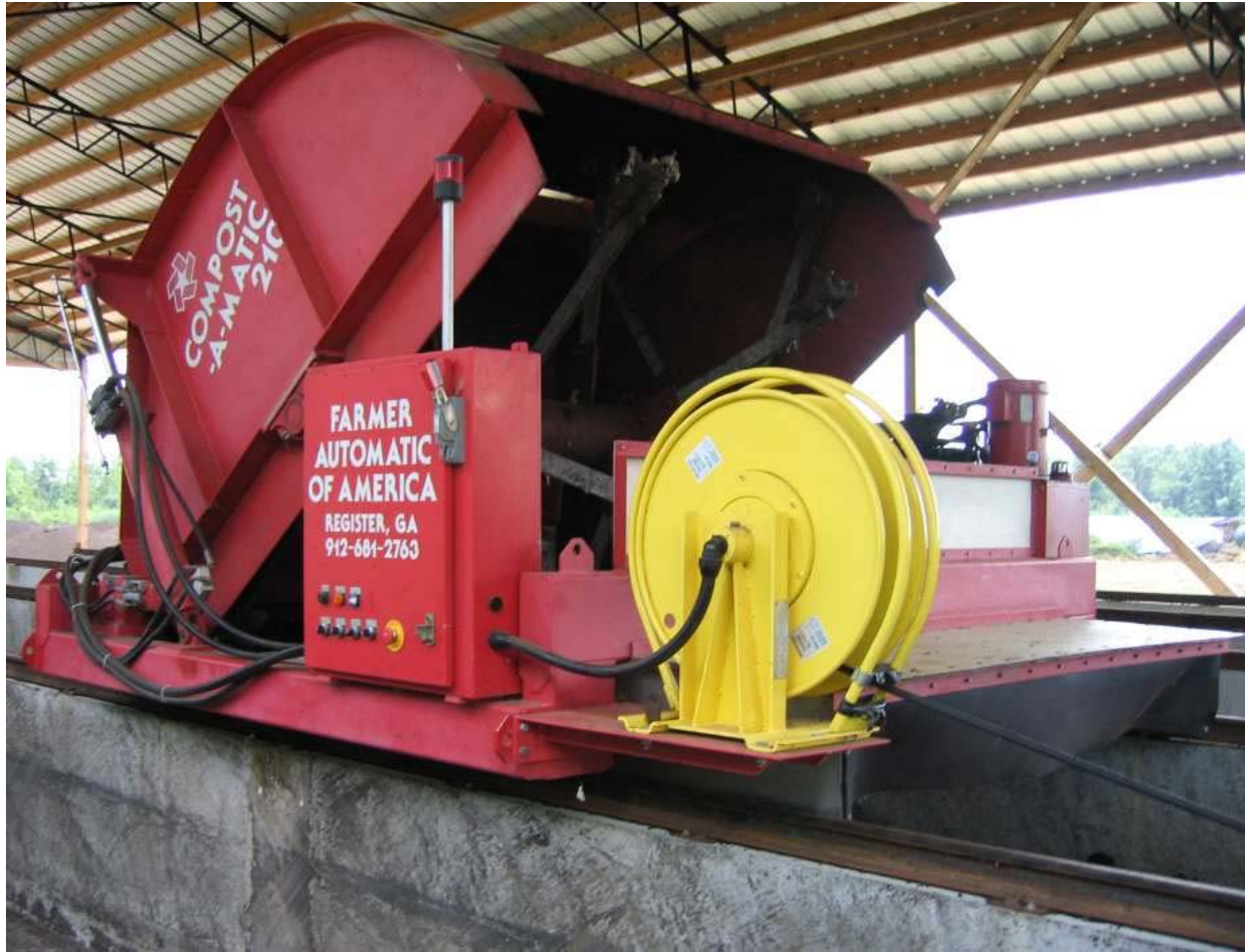
Figure 4.4 Close-up view of mechanical mixer used to mix compost.
