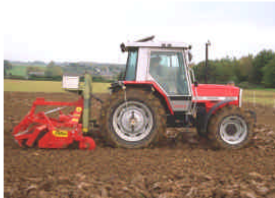
Figure 5.3 Measurements of draught, torque and pto speed for a rotary cultivator
