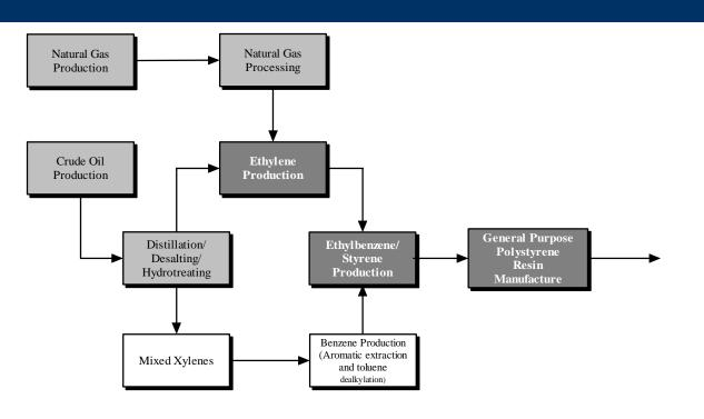
Flow diagram for the production of general purpose polystyrene resin. Shaded boxes represent recently updated data for the US LCI Database. Darker boxes with white text represent data expected from APC member.
