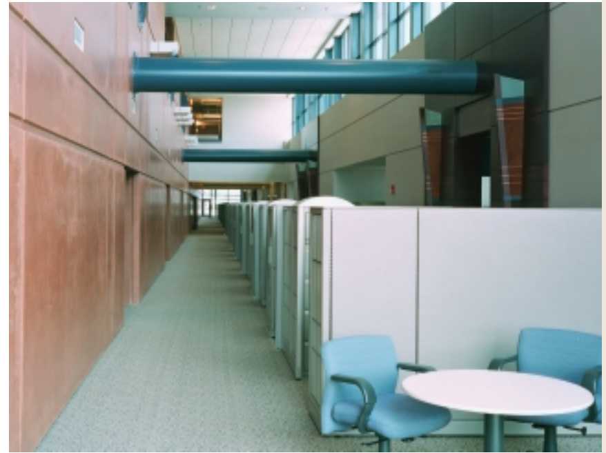
Clerestory windows provide natural daylighting to open bay offices.
