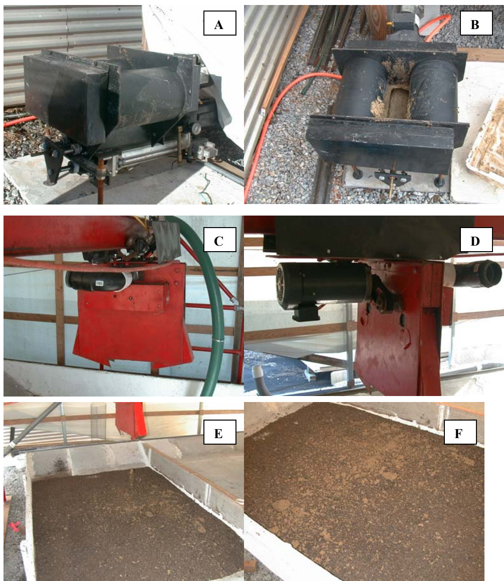
Figure 4. Compressed air driven piston pump (A and B) was used to deliver fresh manure to a manure spreader traveling a beam (C and D). Shielded rotating fans spread the manure across the larval basin (E and F).
