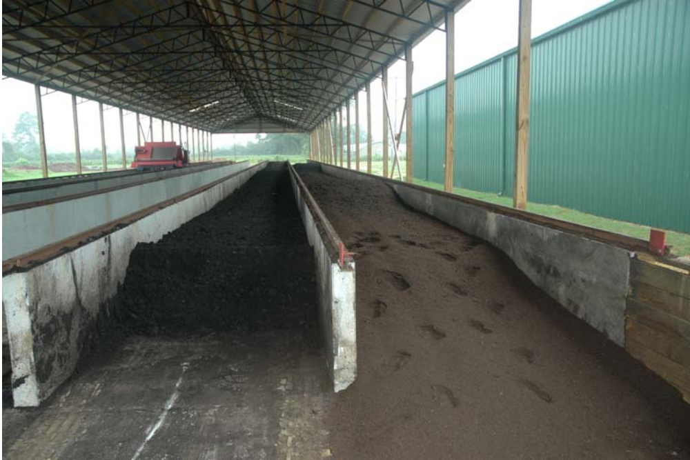
Figure 7: Composts at the end of the bins. Bin #1 (left) used a mixture 1SS:2CGT:4WC, and bin #2 (right) used a mixture 1SS:2CGT (SS=separated manure solids, CGT=cotton gin trash, and WC=wood chips).
