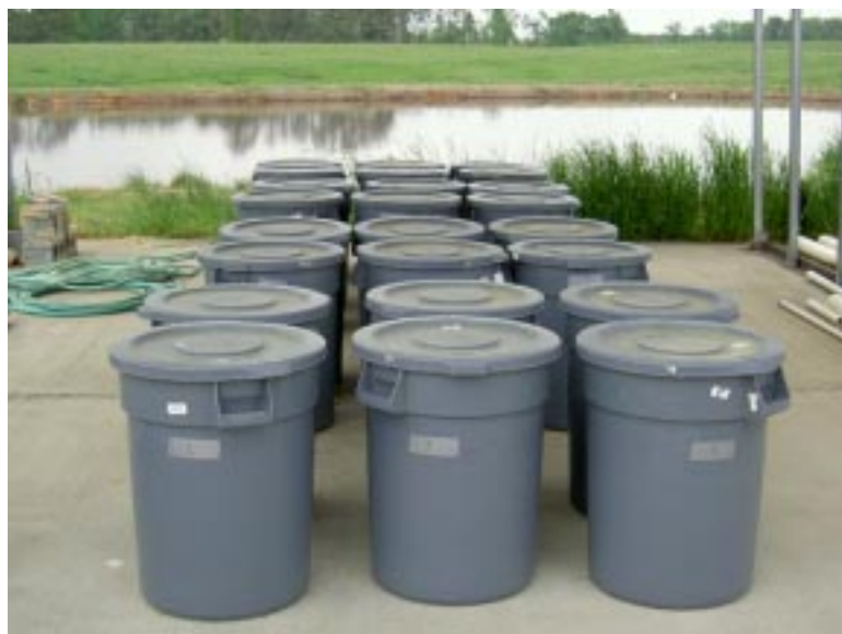
120-liter opaque plastic containers were used to simulate anaerobic waste treatment conditions.
