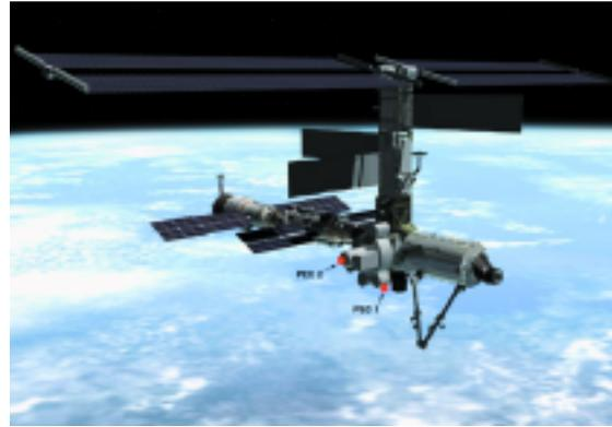
**Figure 9. Location of Two Passive Experiment Carriers (PECs) on International Space Station.**
