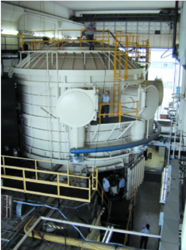
**Figure 3. An Outside View of LHMEL's Cryogenically-Shrouded Vacuum Chamber.**
