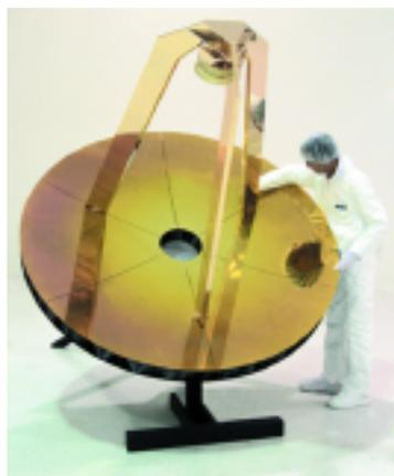
**Figure 8. A 2-Meter Polymer Matrix Composite Mirror Produced for NASA JPL.**
