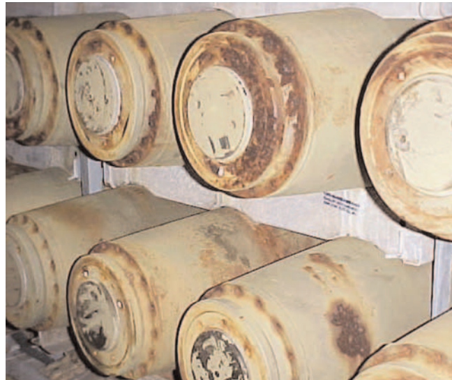
Figure 5. Munitions Are Frequently Stored in High Humidity Environments.
