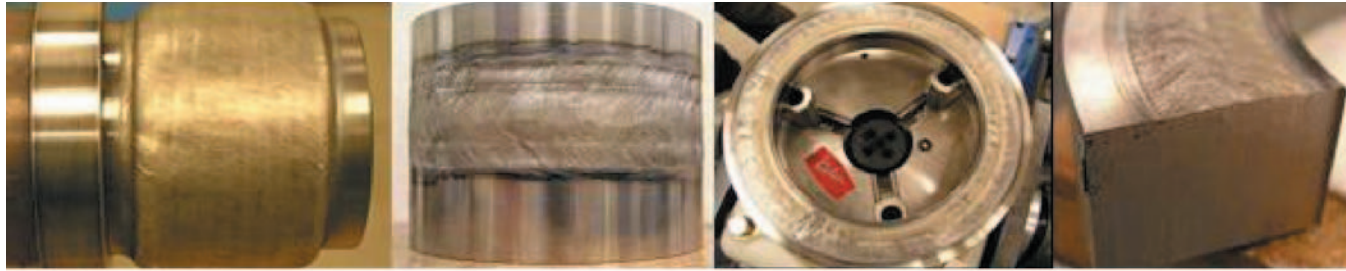
Figure 9. Cladding Results Using RLC with Strip Feeder.
