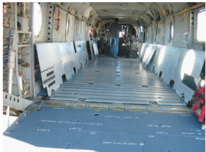
Figure 8. BPS Installation in an MH-47 Chinook Helicopter.
