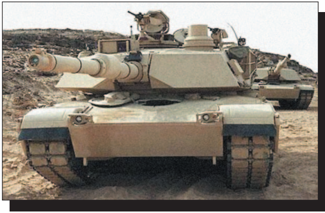
Figure 5. The M1A1 Abrams Tank’s Main Armament: The 120mm M256 Cannon.
