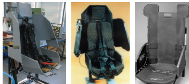
Figure 2. Helicopter Seats[i]: European Tiger Helicopter Seat, Cercom Inc. (Left); AH64 Apache Helicopter Seat Using Hot-Pressed Boron Carbide, Simula Inc. (Middle); and MH-60 Blackhawk Seat, Ceradyne Inc. (Right).
