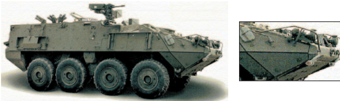
Figure 3. Stryker Combat Vehicle Mounts a Licensed Version of the MEXAS™ System† and is Based on the Light Armored Vehicle 3rd Generation (LAV III) Chassis and Hull. General Dynamics Land Systems – Canada[ii].
