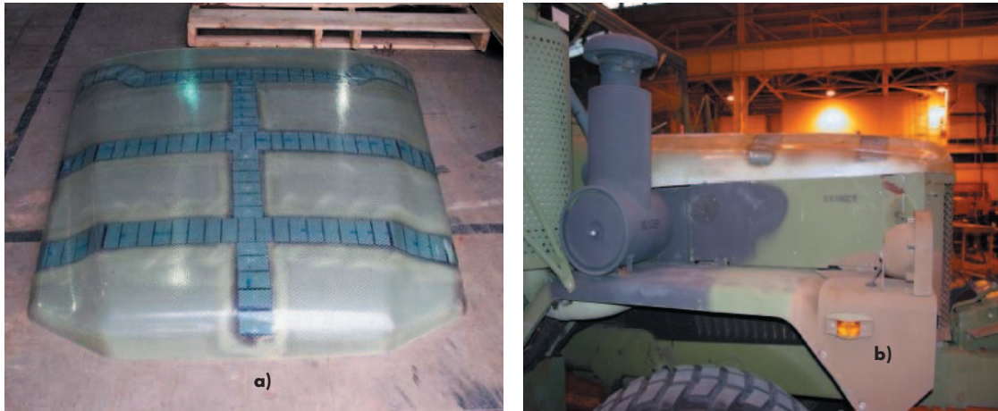
Figure 6. Photographs of a) the Unpainted Composite Hood and b) the Hood Affixed on an M35-A3 Truck. The Blue Stripes are PVC Foam Stiffeners that are Fabricated into the Part.
