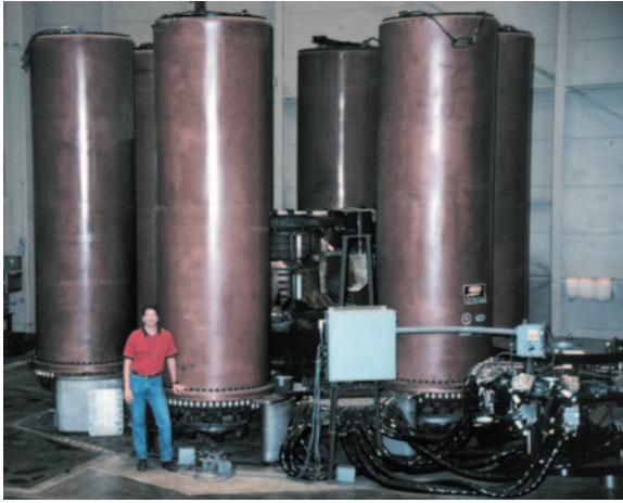
Figure 2. Homopolar Generator (1985) and Subscale Compulsator (1998) Developed under Army Contracts at the Center for Electromechanics, the University of Texas in Austin.
