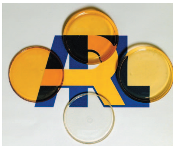
Figure 3. Transparent Nanocomposite Materials That Have Demonstrated Increased Hardness Suitable for Scratch Resistant Coatings.
