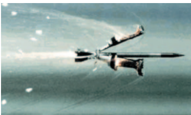
Figure 7. A Sabot Falling Away from a Projectile After Firing.
