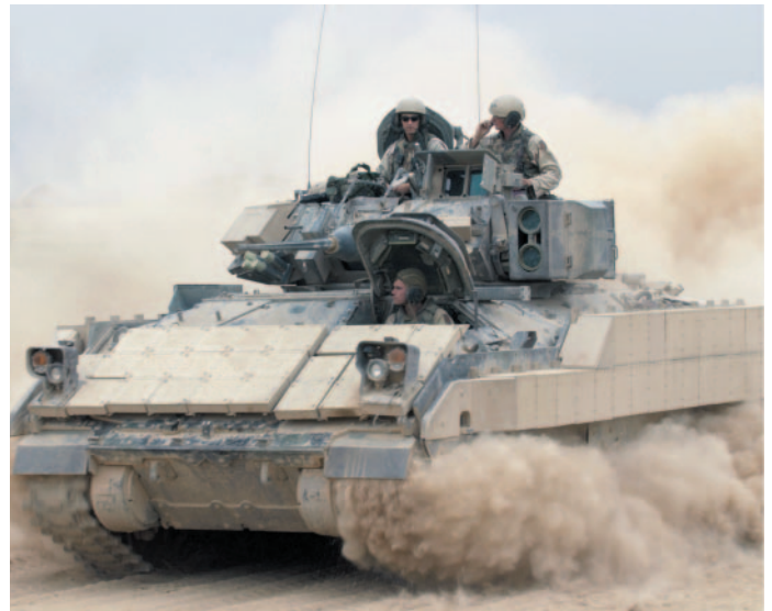
Figure 3. The Bradley Fighting Vehicle Makes Use of Both 7039-T64 (Upper Half) and 5083-H131 (Lower Half).
