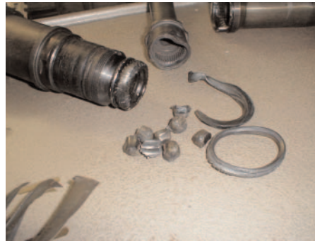
Figure 2. Yielding Failure of UH-1 Helicopter Engine Shaft and Bearing Components[2].
