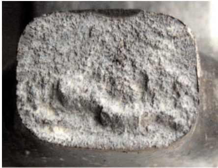
Figure 1. Brittle Fracture Surface of a High-Strength Chain. Fracture Began in a Small Crack Resulting from a Heat Treating Problem (Photo Courtesy of Sachs, Salvaterra & Associates, Inc.).
