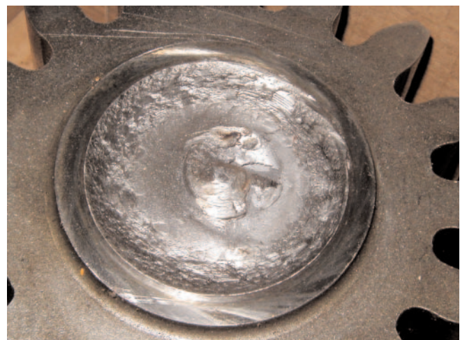
Figure 8. Torsional Low-Cycle Fatigue Fracture of a Shaft. (Photo Courtesy of Sachs, Salvaterra & Associates, Inc.)
