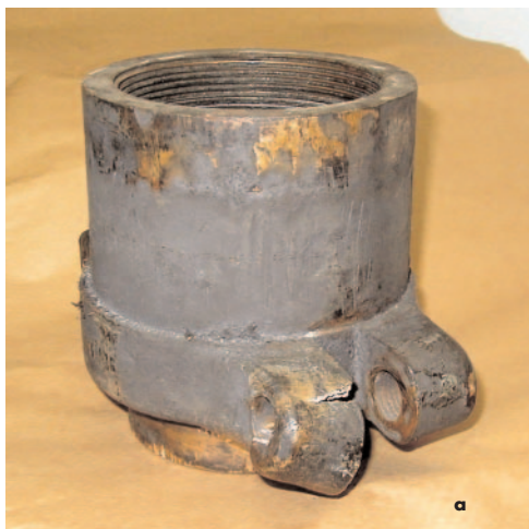
Figure 3. (a) Ductile Fracture of 2 1/2 Inch Hose Fitting (b) Close-up of the Deformed Region Where a Pin Joining the "Ears" Became Free from the One on the Right Causing the Deformation and Fracture of the One on the Left (Photos Courtesy of Sachs, Salvaterra & Associates, Inc.).
