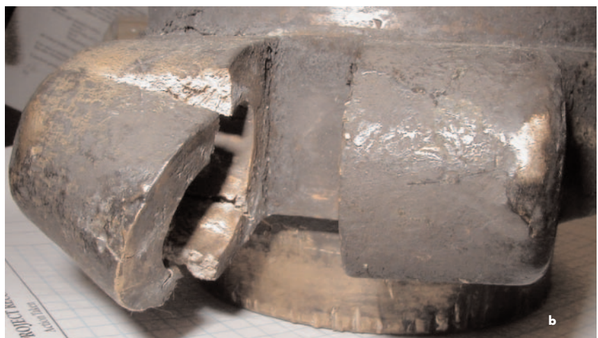
Figure 3. (a) Ductile Fracture of 2 1/2 Inch Hose Fitting (b) Close-up of the Deformed Region Where a Pin Joining the "Ears" Became Free from the One on the Right Causing the Deformation and Fracture of the One on the Left (Photos Courtesy of Sachs, Salvaterra & Associates, Inc.).
