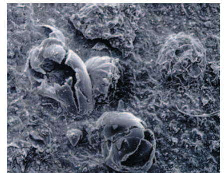
Figure 4. Tubercles as a Result of MIC (Courtesy of Metallurgical Technologies, Inc.) [9].
