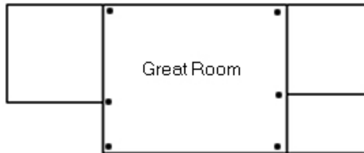
Figure 17. Definition of vertices for typical floor plan
