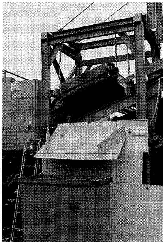
Figure 14 Magnetic belt used to remove metal from waste reroofing shingles
