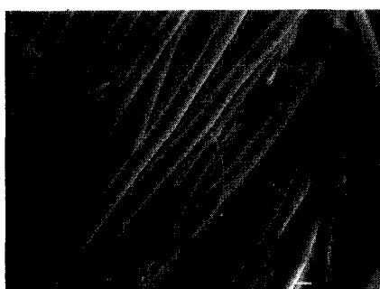
Fig. 2. Surface modification of lyocell of untreated (left) and cellulase treated (right), as viewed by SEM at 100X magnification.
