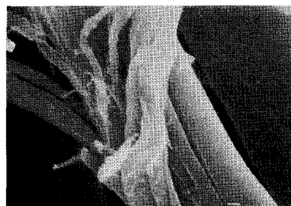
Fig. 3. Lyocell fiber showing primary fibrillation as viewed by a SEM at 500X magnification.
