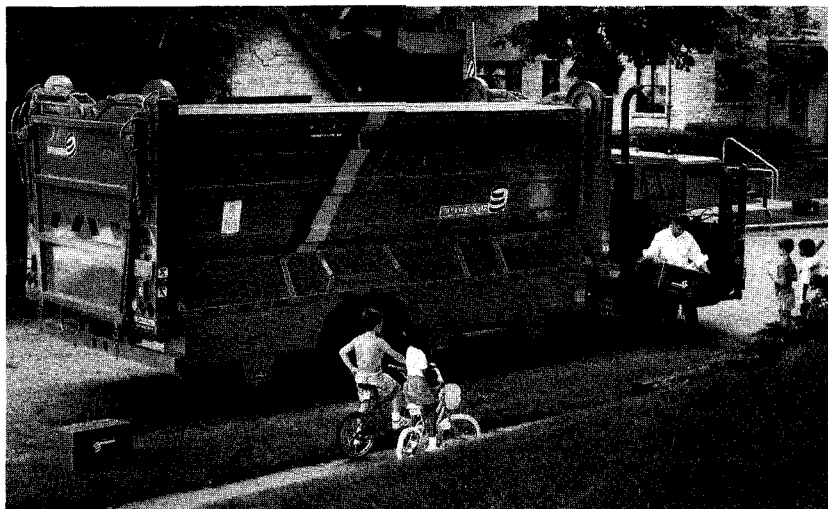
A side loading or "over the top" recycling vehicle minimizes loading fatigue for the crew. (Photo courtesy of Dempster, Toccoa, GA.)
