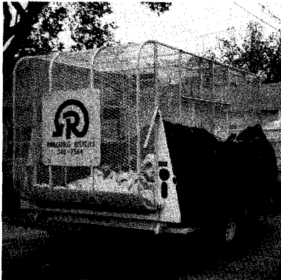
(Left) A simple solution is adding a trailer to the back of a recycling vehicle. Because the trailer was added, the vehicle can haul larger amounts of plastic soda bottles and milk, juice, and water jugs. (Photo courtesy of Dan Krivit and Associates, St. Paul, MN.)
