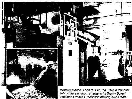
losses to a low 2-3%, compared to 10-15% that would occur with reverb melting.
