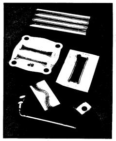
*Figure 2.* Parts hardened by direct resistance heating.
