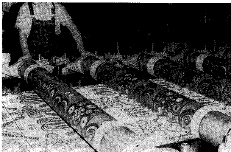
Fig. 3. Printing with electroformed nickel screen-printing cylinders. (Photo courtesy of Nickelmesh AG, Rudolfstetten, Switzerland.)
