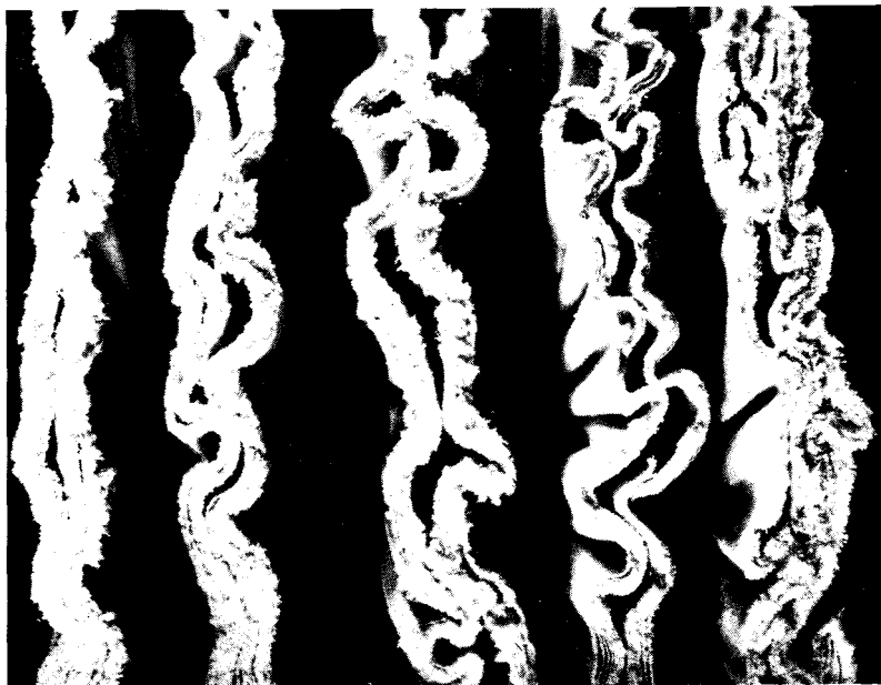
Fig. 6. Cloth bias buffs in order of increased density from closed face (left to right: 0, 2, 4, 6) to open face (far right) design.
