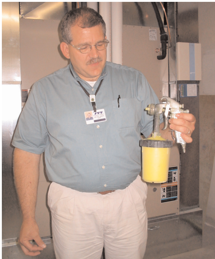
Facilities manager, Bryan Urban, displays new siphon-fed coatings gun system.
