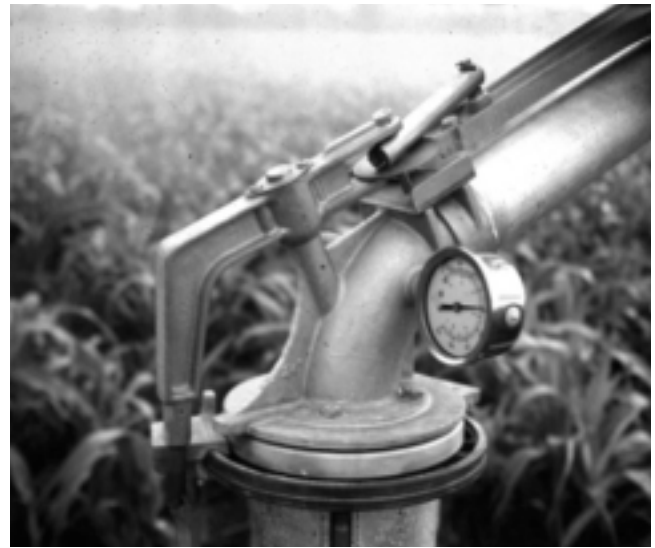
Figure 8. Pressure gauge installed on a traveling gun.
