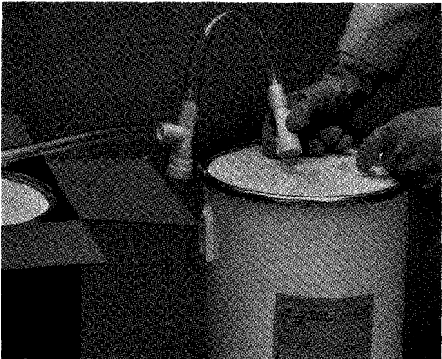
Disconnect the circulating unit from the outlet side of the cartridge.
