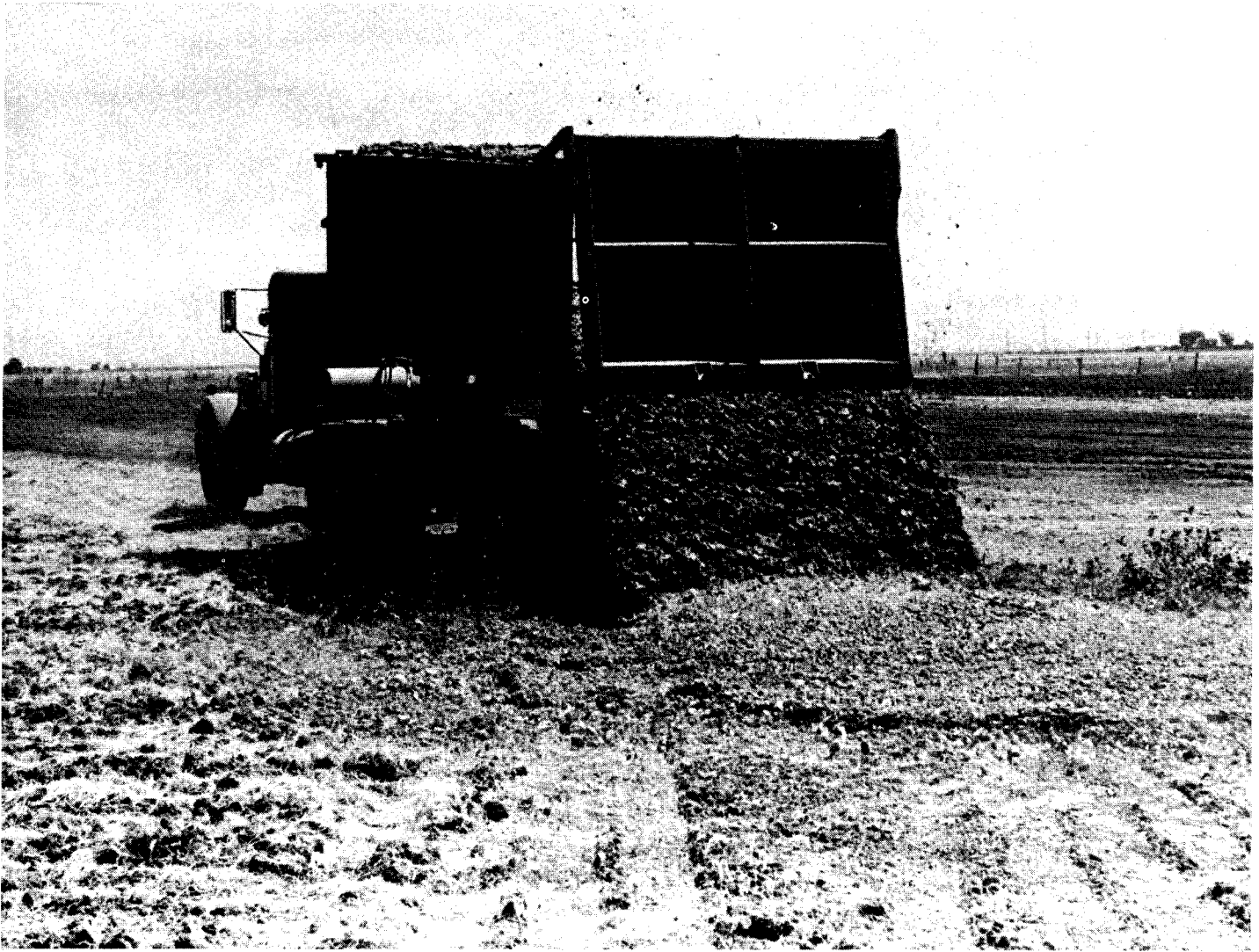
Figure 5.15. Discharging residuals evenly — an important step.
