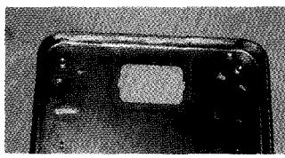
2. Good cleaning but poor phosphate development; light phosphate coating and low pH, producing pickling of metal substrate
