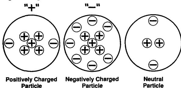
A neutrally charged particle has an equal number of protons (positive charges) and electrons (negative charges). A negatively charged particle has more electrons than protons. A positively charged particle has more protons than electrons.
