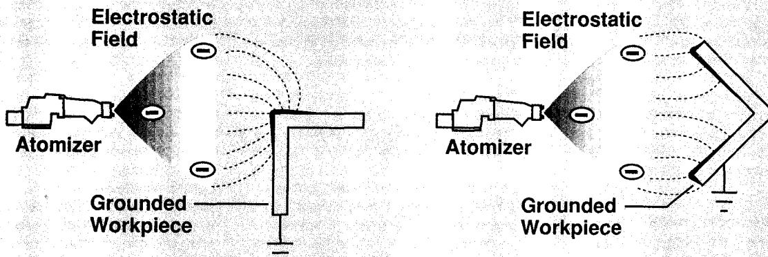
Paint particles are attracted to the edges of a workpiece while avoiding inside corners and recesses.
