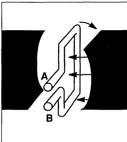
No electricity is generated in the loop in this diagram because the wire does not cut through the lines of force.
