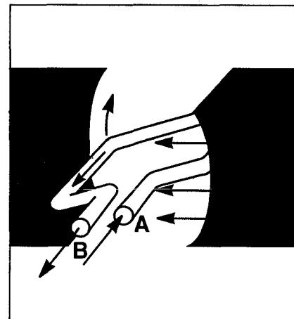
The current reverses as the wire makes the second half of the turn. The current flows from point A to point B.
