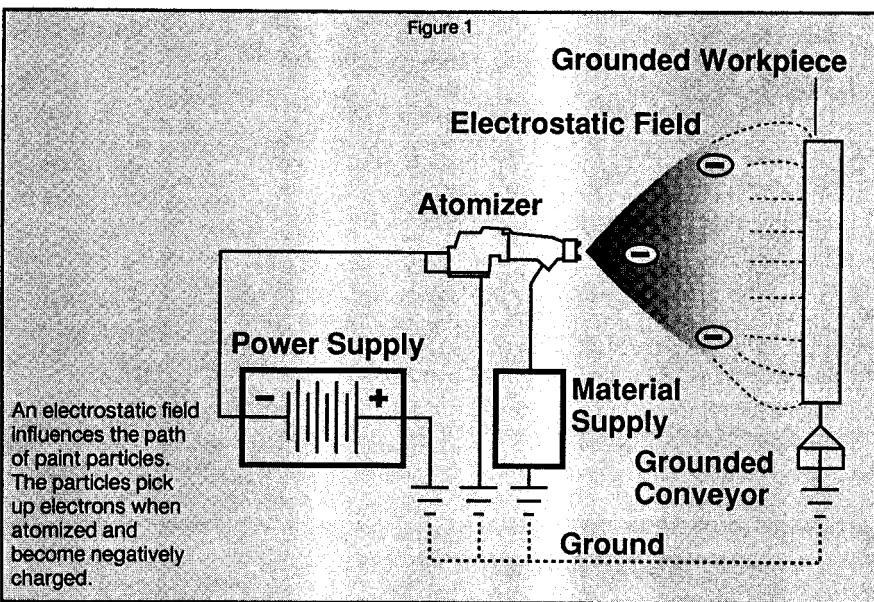
currents. Large particles sprayed at high speed have great momentum, reducing the influence of the electrostatic force. A particle's directional force inertia can be greater than the electrostatic field. Increased particle momentum can be advantageous when painting a complicated surface, because the momentum can overcome Faraday cage effect (the tendency for charged paint particles to deposit only around the entrance of a cavity) (Figure 2).
