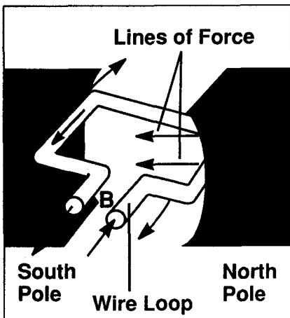
The current flows from point B to point A through the loop when the wire is rotated clockwise, as shown above.
